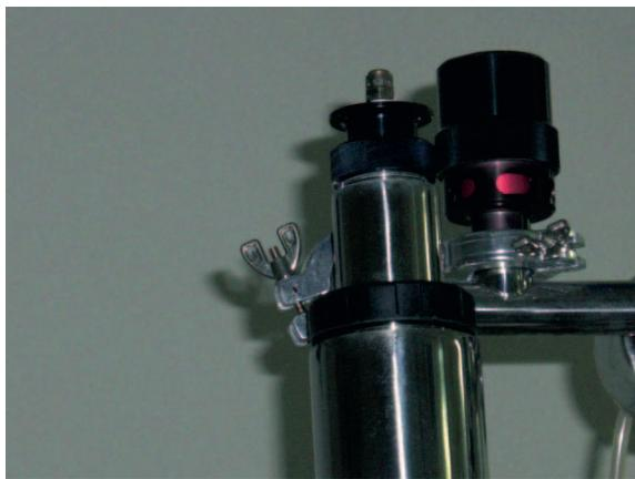
**Fig. 1** - Plug valve which, upon reaching a maximum pressure value, and in case of overheating of the magnet, opens, releasing helium into the environment.
