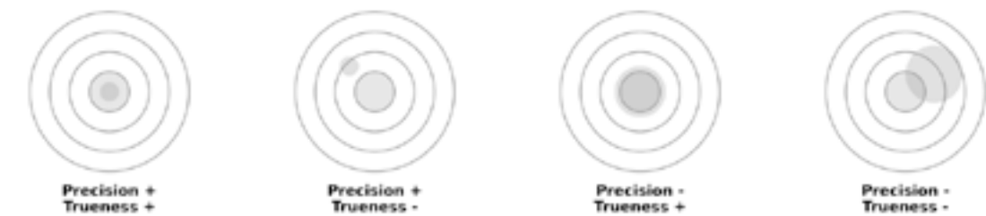
Figure 2. Graphical representation of the two components of accuracy: trueness and precision. Adapted from Dr. Jan-Frederik Gürh, University of Munich).
